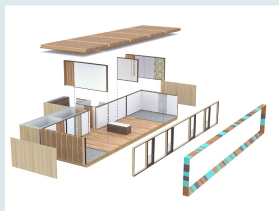
Figure 6.11 - Exploded axonometric view of the UMAR module (copyright Werner Sobek, Stuttgart/Germany)
